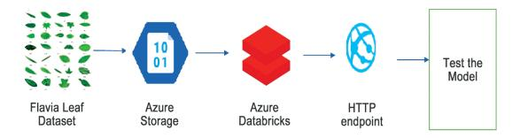
The Azure Databricks which is an Apache Spark-based analytics platform is the key solution for the given architecture. It integrates with Azure services such as Azure storage and provides efficient analytic solutions for end user.
